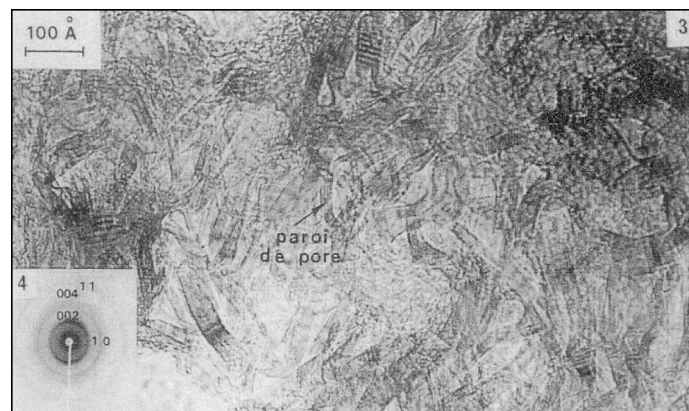
Figure 1. Lattice-fringe image of Oklo sample 8 (previously heated to 2800 °C) reveals onion-skin structure and small size of pores and their lack of flattening. Diffraction pattern (lower left) shows diffuse (002) arcs, imparting slight statistical orientation of basic structural units in this organic matter (paroi de pore = partition wall of pore) (after Cortial et al., 1990, p. 79, Plate I, Fig. 3).
